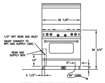
ELECTRICAL CORD LOCATED IN BACK OF UNIT LOCATION OF ELECTRICAL OUTLET MUST NOT BE HIGHER THAN 3" FROM FLOOR IF LOCATED BEHIND THE UNIT OR CAN BE LOCATED IN AN ADJOINING CABINET.
